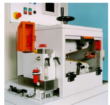
The infeed belt can work in both parallel and nip modes. The distance from the belt to blade is 40 mm.
